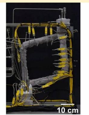
Fig. 3. Side view of a completed microloop installed into its test stand.
